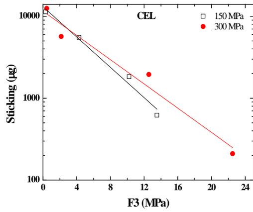
**Fig. 1.** (a) Cohesive strength of CEL and IBN at different compaction pressures, (b) relationship between sticking and F3 for CEL.
